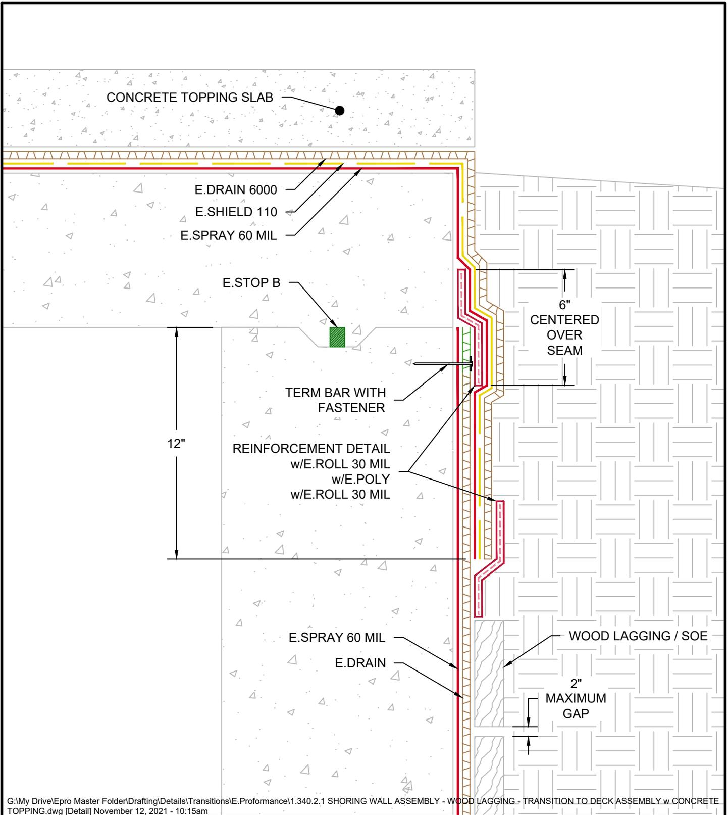
SHORING WALL ASSEMBLY - WOOD LAGGING - TRANSITION TO DECK ASSEMBLY w/ CONCRETE TOPPING
